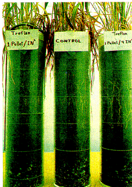
Various concentrations of the herbicide trifluralin (Treflan) were tested against controls to determine the best concentration for stopping unwanted root growth.
